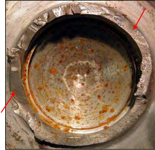
Figure F1: Macro image of fracture surface of shear pin 11. Two distinct areas of fatigue are seen on the fracture surface (indicated with red arrows). Image taken with oblique angle lighting to emphasize fatigue zones.
