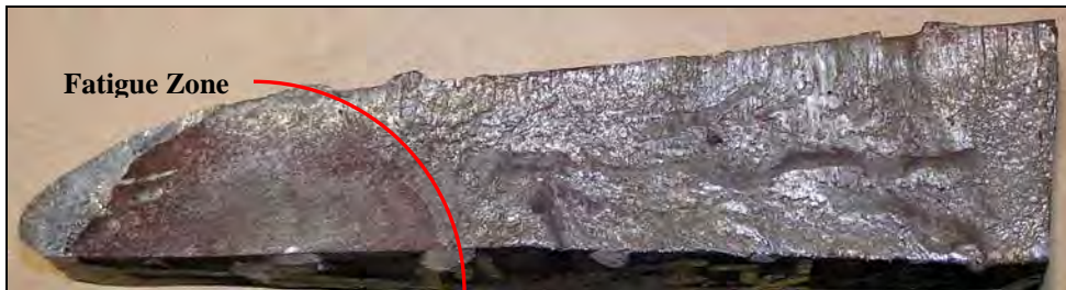
Figure F7: Macro image of sample removed from blade 14
