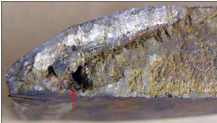
Figure F12: Macro image of large subsurface weld defect (indicated by red arrow).
