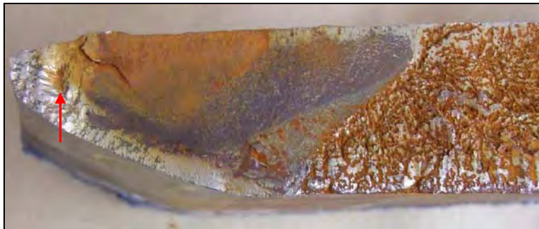
Figure F10: Macro image of fatigue crack portion of blade 2 fracture surface showing striations and subsurface weld defects (indicated by red arrow).
