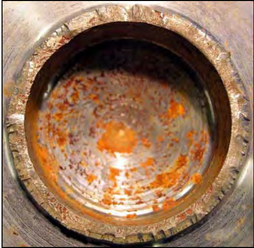
Figure F4: Macro image of fracture surface of shear pin 13.
