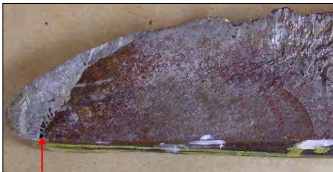
Figure F8: Macro image of fatigue crack portion of blade 14 fracture surface showing striations and subsurface weld defects (indicated by red arrow).
