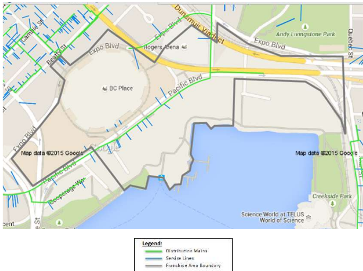
Figure 3: Map of Distribution Mains and Services available to Serve NEFC Area Customers
