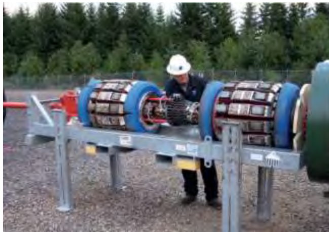
Figure 3-8: Typical EMAT Tool 12
